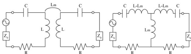
(a) Equivalent circuits of magnetic resonant coupling of two antennas
