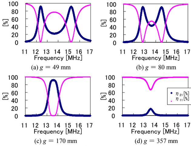
Fig.4. Results of electromagnetic field analysis for efficiency vs. frequency at different gap lengths.
