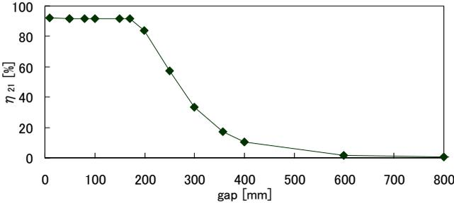
Fig.5. Results of electromagnetic field analysis for peak efficiency vs. air gap length.
