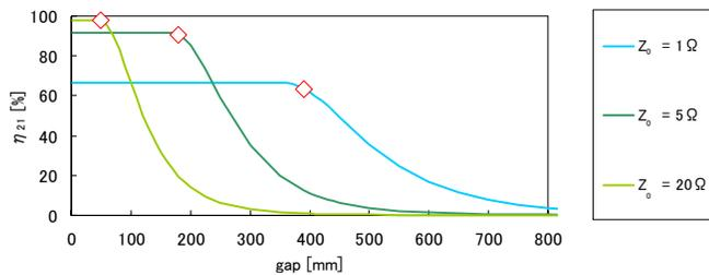
Fig.11. Peak efficiency at each gap length related to characteristic impedance. Dots are the boundary conditions at maximum efficiency.
