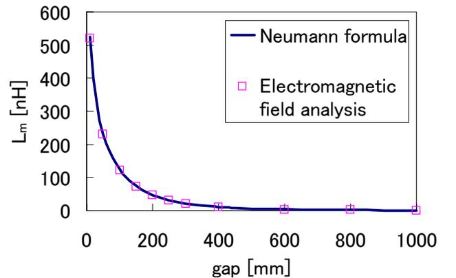
Fig.7. Optimized parameters of mutual inductance and characteristic impedance in relation to maximum efficiency for different air gap lengths.
