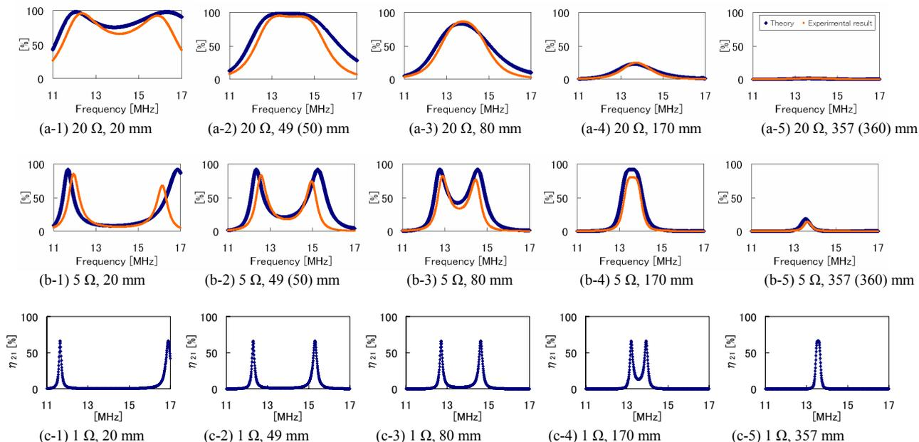
Fig.9. Efficiency and frequency at characteristic impedance and different air gap lengths using equivalent circuit and experimental results.
