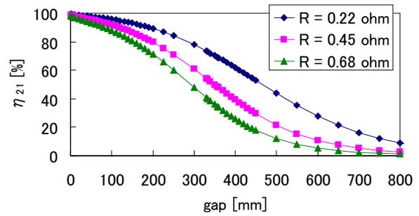
Fig.14. Maximum efficiency vs. air gap length for internal resistances.
