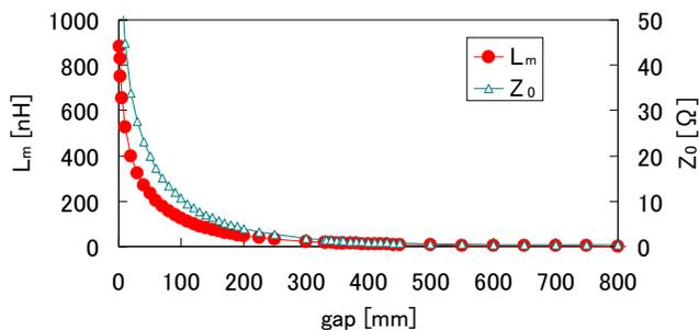
Fig.13. Optimized parameters of mutual inductance and characteristic impedance with maximum efficiency at each air gap length.
