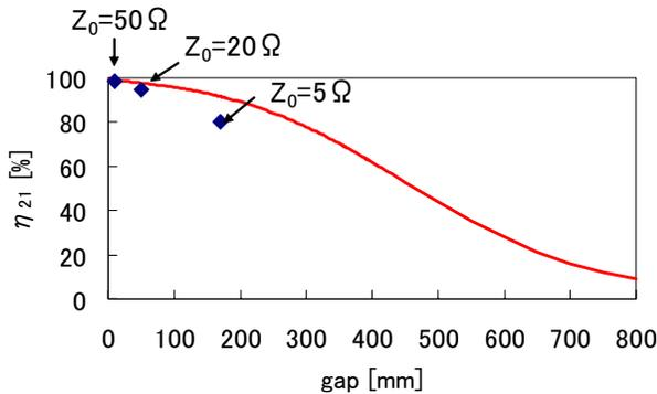
Fig.12. Maximum efficiency vs. air gap length.
