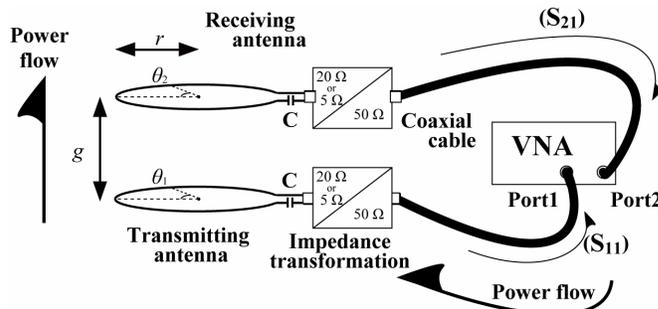
Fig.2. Parameters of helical antennas and experimental setup.
