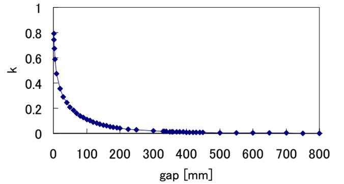
Fig.6. Coupling coefficient  $k$  vs. gap length.
