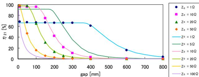
Fig.10. Peak efficiency for each gap length related to characteristic impedance. Dots denote the results of electromagnetic field analysis, and lines denote the theoretical results based on equivalent circuits.
