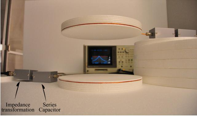
Fig.3. Photograph of experimental setup. ( $g = 170$  mm)
